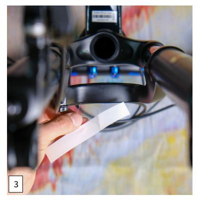
To apply the paint protection strips, remove the front wheel and clean the inside of the suspension fork with a cloth and a suitable cleaner (see picture 1).
