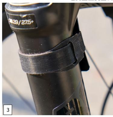
After preparation, the mudguard is pre-assembled to determine the length of the Velcro straps for attachment to the triple clamp.
