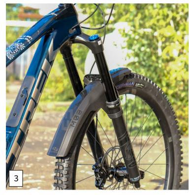
Finally, the mudguard is pushed in again and all Velcro ties are tightened (see pictures 1 and 2)
